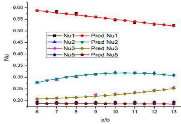
Figure A7. Comparison between predicted function and CFD results for Nusselt number of the blocks at bar position  $y=5.5b$ ;  $a=b$ ,  $Re=50$
