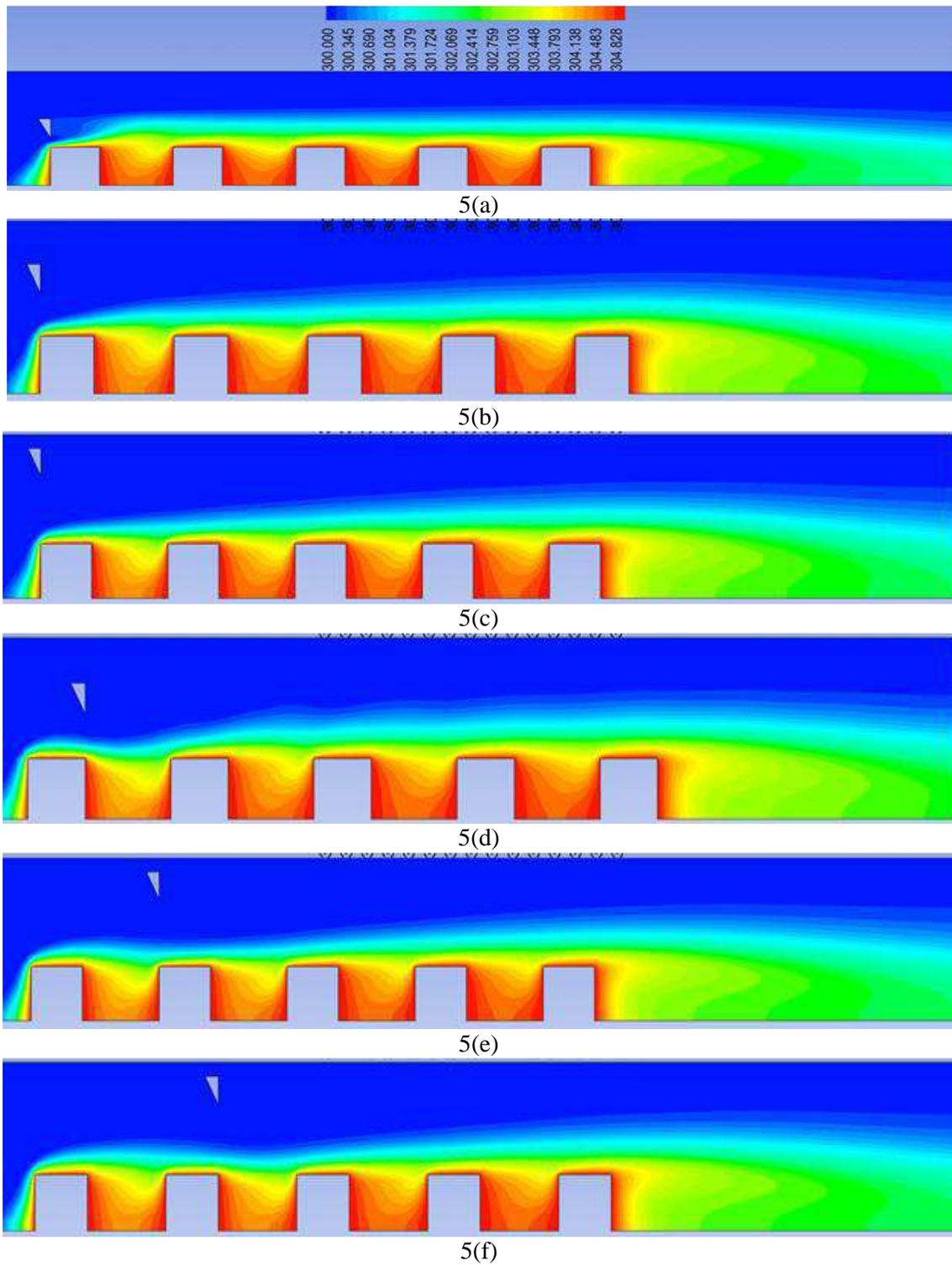
Figure A5.Deviation of temperature contours with alteration of bar location fixing  $Re=200$  (a)  $x/b=6$ ,  $y/b=3.5$ , (b)  $x/b=6$ ,  $y/b=4.5$ , (c)  $x/b=6$ ,  $y/b=5.5$ , (d)  $x/b=8$ ,  $y/b=4.5$ , (e)  $x/b=11$ ,  $y/b=5.5$ , (f)  $x/b=13$ ,  $y/b=5.5$
