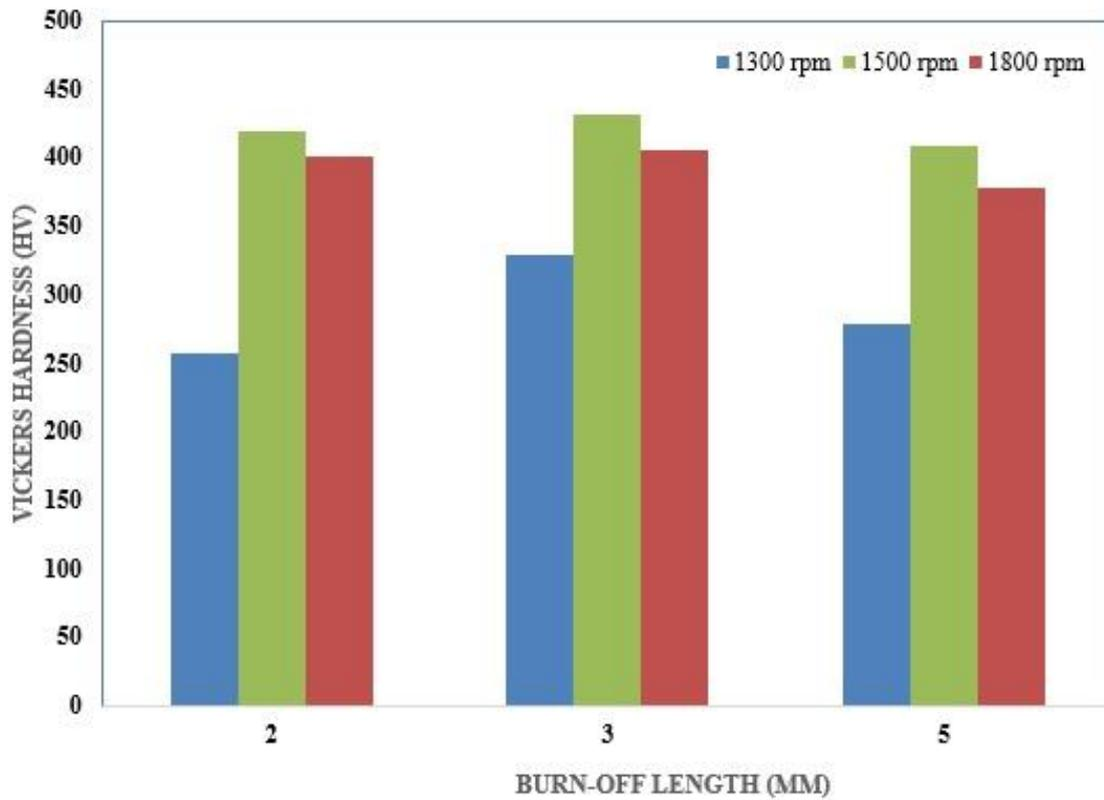
Figure B2. Variations of micro hardness with rotational speed and burn-off length
