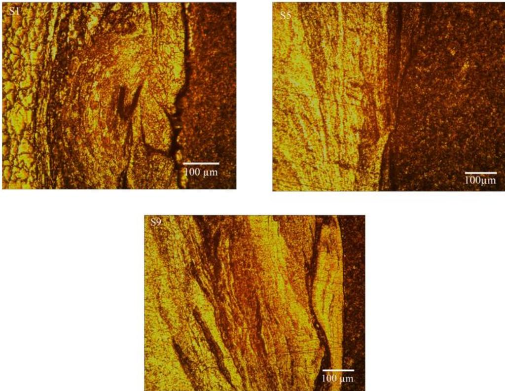
Figure B3. Microstructures at interface region for all samples S1, S5 & S9
