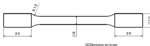
Figure 2. Tensile specimen dimensions
