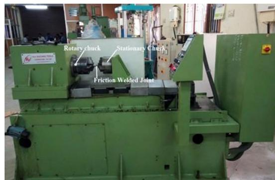
Figure 1. Friction welding machine
