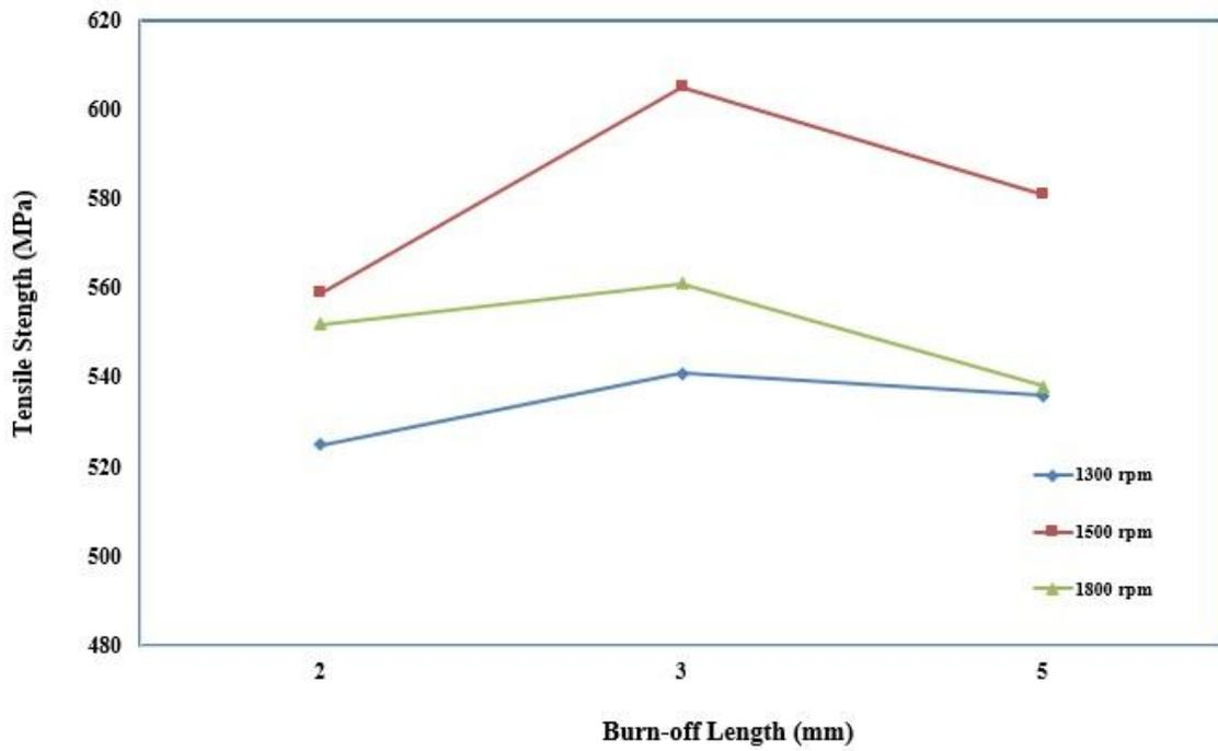
Figure B1. Variations of tensile strength with rotational speed and burn-off length
