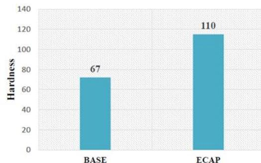
Figure 2. Comparison of microhardness test
