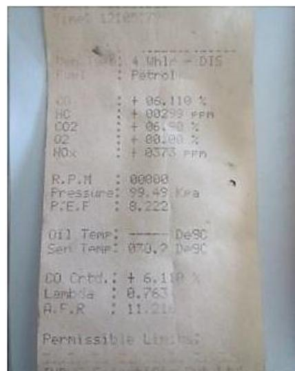
Figure 4. Exhaust gas result after 10 minutes of engine operation
