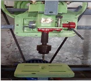
Figure 3. Drilling centre through bevel gear arrangement
