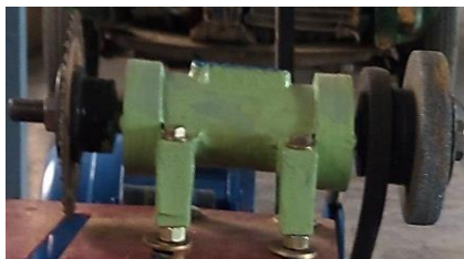
Figure 4. Grinding and circular saw cutter- belt drive arrangement
