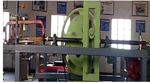
Figure 5. Sawing/ cutting and slotter end operations using scotch yoke mechanism
