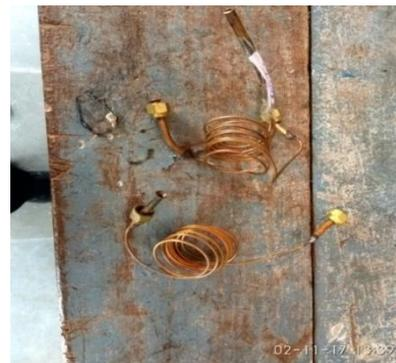
Figure 6. Capillary with end tubes
